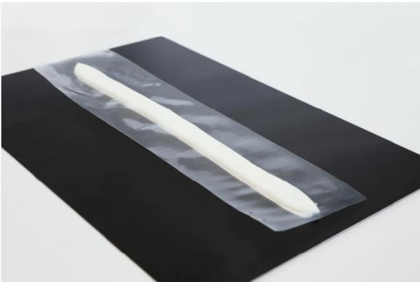
Pic 3: Press bead down to half height
