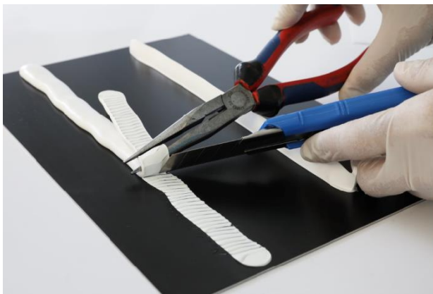
Pic 5: Turning the bead to get maximum tension and cut
