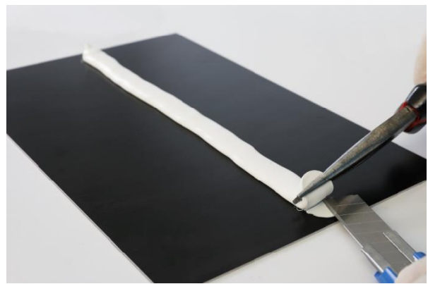
Pic 4: After full curing separate first 3 cm of the bead
