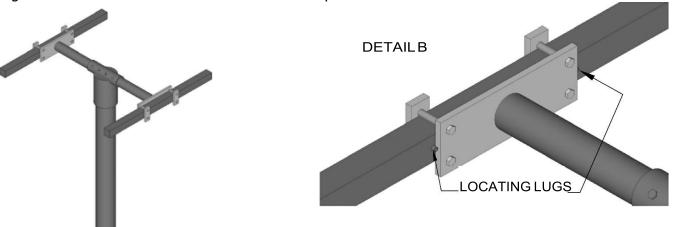
Slide cross pieces into flat bar arrangement. Make sure locating lugs on cross pieces are facing in. See Detail "B" of locating lugs.
