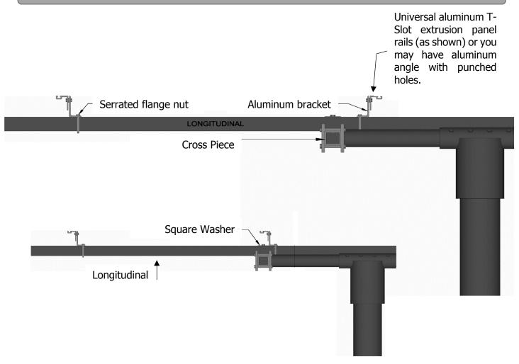
Bracket orientation in most installations is generally opposed to one another as in top picture. It may be necessary to have brackets facing in same direction as in bottom picture, if panel size is such that you need to do this to maintain a ¼" gap between panel ends on centerline.
