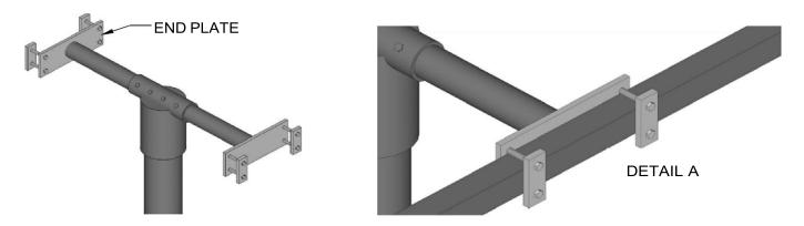
Finger tighten onto "Tee" end plates aluminum flat bar and straight 1/2" bolts. Place entire "Tee" assembly on top of post. The aluminum flat bar and straight 1/2" bolts are shown in Detail "A". Tighten both set bolts and the four bolts on the top of the "Tee".
