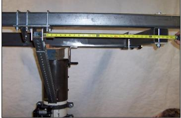
Insert 7/16" bolt through lugs and upper end of telestrut and tighten. Make sure middle bolt is installed through telestrut in the hole that is circled, tighten nyloc onto bolt.
