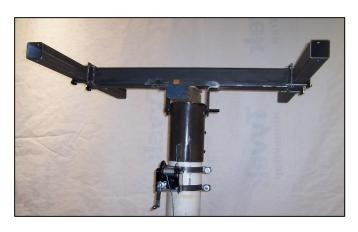
Install 2 cross pieces. Make sure small socket head bolts reference either side of center tube end plates. Leave 5/8" x 6" clamp bolts just slightly less than tight to facilitate installing longitudinals in next
