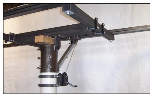
Wind up all the slack. Then it is safe to remove wedges and wood block.
