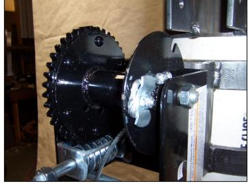
Bolt winch to foundation/bracket with  $3 - \frac{1}{2}$ " bolts. **DO NOT** cut plastic zip ties holding cable yet. Install handle.
