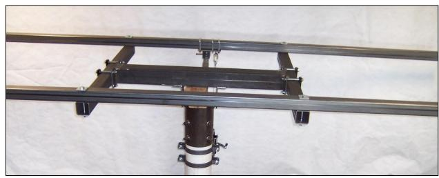
Move the longitudinals as close as possible to horizontal to one another to begin installing rails. 15X and 18X use channel rails and have no brackets. 12XHD uses angle rails and brackets to attach rails to the longitudinals.
