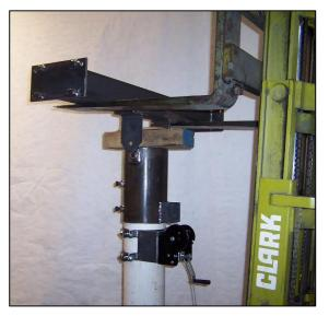
Place 4" block of wood on top of pivot cap. Keep 2 wedges handy. This block **MUST NOT BE REMOVED** until telestrut, winch and cable are installed and fully secured. **Severe injury may result if center tube pivots without block or telestrut/winch restraining or controlling it!**
