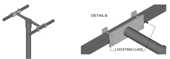
Slide cross pieces into U-Bolts or bolt and flat bar arrangement. Make sure locating lugs on cross pieces are facing in. See Detail "B" of locating lugs.
