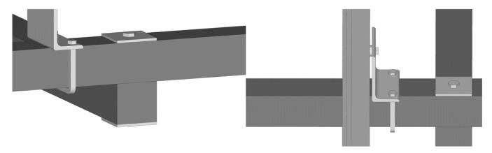
**General view of assembly**. When fastening panels to rails, place first panels at end of rails marked "TOP" and work down until all panels are in place with bolts finger tight. Cross measure array for square, check to see that all spaces (approx. ¼") between panels are equal, then tighten all bolts.
