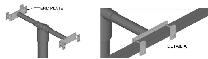
Finger tighten onto "Tee" end plates, either the U-Bolts or aluminum flat bar and straight 1/2" bolts, whichever come with your mount. Place entire "Tee" assembly on top of post. The aluminum flat bar and straight 1/2" bolts are shown in Detail "A".
