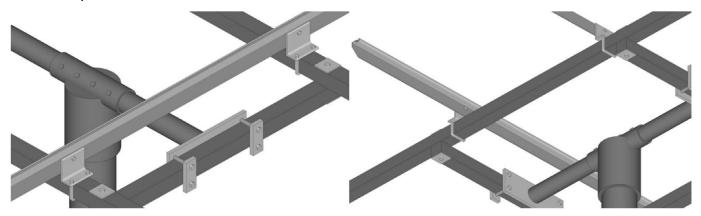
Attach aluminum rails as shown. If rail ends are marked "TOP", align them to the same end.
