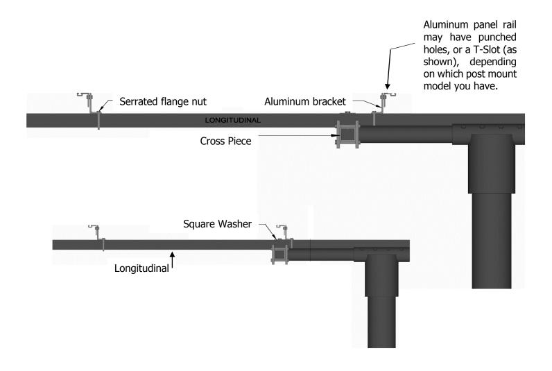
Bracket orientation in most installations is generally opposed to one another as in top picture. It may be necessary to have brackets facing in same direction as in bottom picture, if panel size is such that you need to do this to maintain a 1/4" gap between panel ends on centerline.
