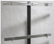
Before you lightly bolt the brackets on to the channels, make sure that the measurements from the OUTSIDE of one bracket to the OUTSIDE of the other bracket on each channel is the same as measurement "A". The smaller brackets go on top and the larger brackets with the "dogleg" go on the bottom channel.
