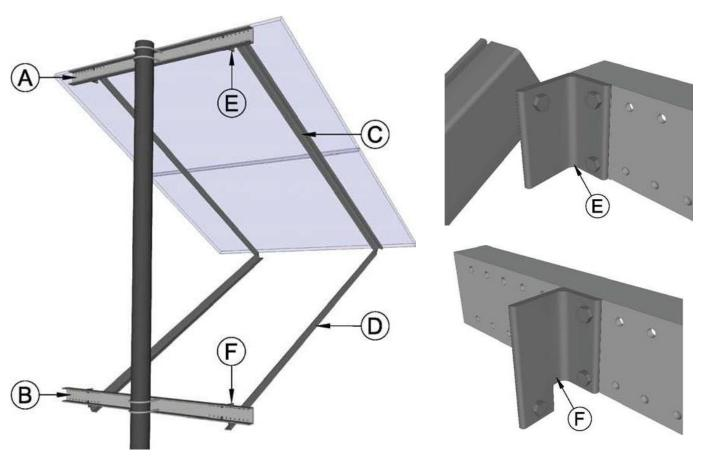
(Two panels shown, punched channel for a variety of module types.)
