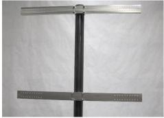
Lightly clamp two channels to your post with the four U-Bolts provided. To determine the approximate spacing between the two channels, use a panel rail to gauge the distance from the top of the top channel to the bottom of the bottom channel.
