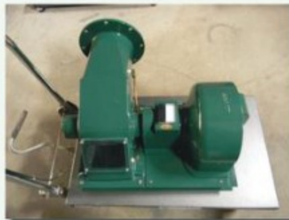
A low-RPM permanent magnet generator is direct-coupled to the turbine.
