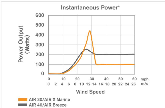
\*Factors affecting turbine output include site turbulence, elevation and air temperature
