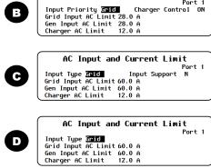
**NOTE:** If multiple parallel inverters are installed with a limited AC source, the combined amperage settings must be less than the AC input circuit. The MATE3s Profile Wizard can perform this calculation. (See page 45.)
