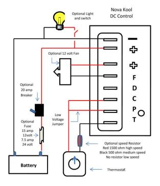
After Serial number 256409 the thermostat wire has an additional green or red wire which is used to control cut out voltage. If it is placed on P the cut out voltage is 9.4 vdc if it is simply left off of terminal P the cut our voltage is 10.6 vdc.
