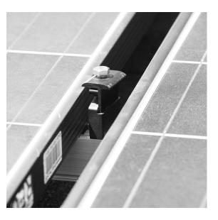
On the outside edge of the last module, install the clamps so that the side with the two stainless-steel pins is on the module frame. Tighten all bolts to the specified torque.
