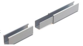
If a cut section of rail is required for the installation, it must not be installed at the end of a row. Each section of rail at the end of a row must be supported by two mounts before being spliced. If a rail section has a splice and 3 roof mounts, the splice should be located within 1/3 rail span of the middle mount.
