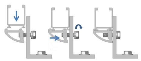
Simply position the adapter into the two feet on the bottom of the rail, and tighten the bolt slightly. Leave the bolt slightly lose to allow leveling of the rails in the next step.
