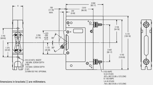
Note: Tolerance  $\pm$  .015 [.38] unless noted. Dimensions in brackets [] are millimeters.
