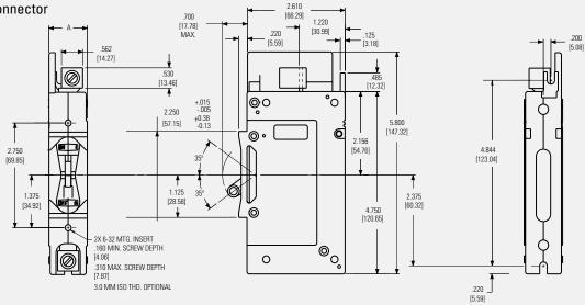
Back Connected Stud Terminal (Front Mounted)
