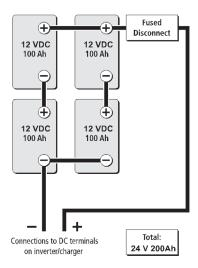
Figure 1-21 Batteries in Series-Parallel Connections
