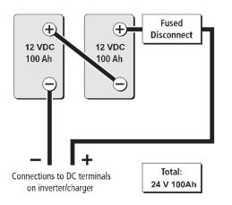
Figure 1-20 Batteries Connected in Series
