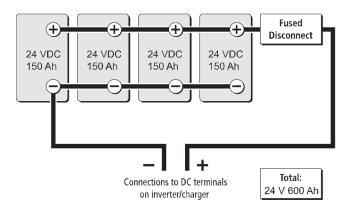
Figure 1-19 Batteries Connected in Parallel
