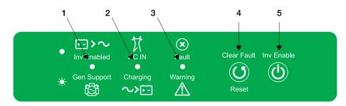
Figure 1-3 Front Panel Buttons and Status LEDs
