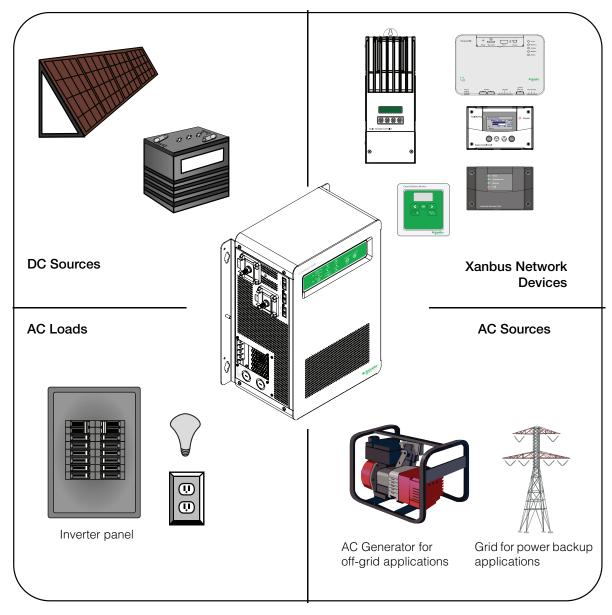
Figure 1-8 AC, DC, and Network Components
