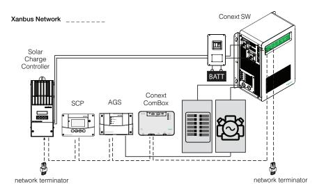
Figure 1-7 Xanbus System Diagram Example
