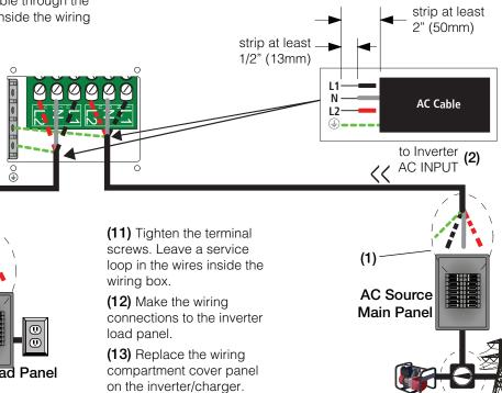
Figure 1-11 Conext SW AC INPUT and OUTPUT Connections
