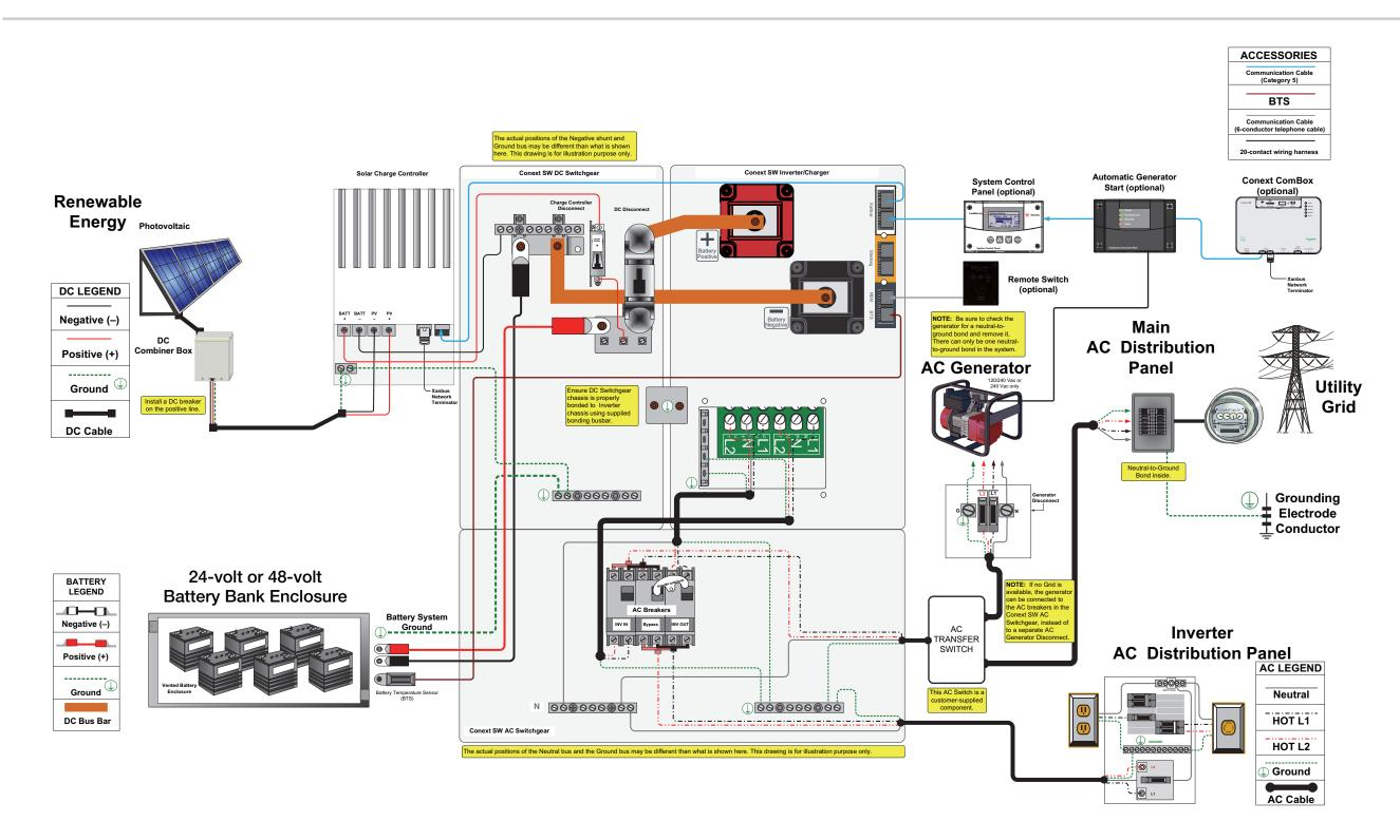
Figure 3-4 Single-Inverter System Renewable Energy (Solar) Wiring
