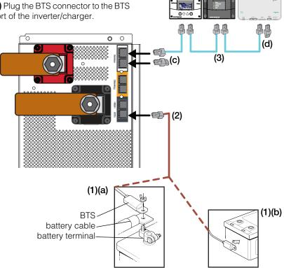
Figure 1-14 Conext SW BTS and Xanbus Connections
