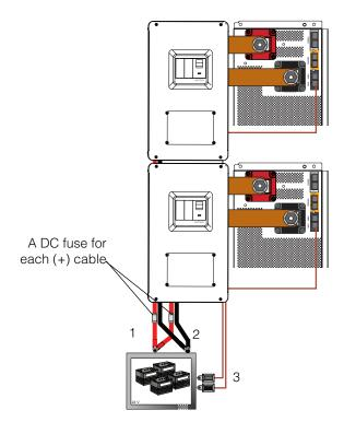
Figure 1-17 Connecting Battery Cables
