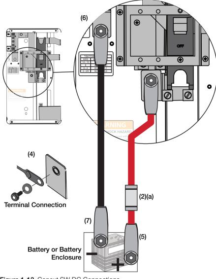
Figure 1-13 Conext SW DC Connections
