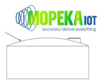
Horizontal Tanks-Install at highest vertical point of tank
