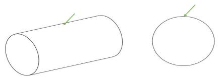
Vertical Tanks- Install in center or on flat area. Do not install on angled surface if angle is greater than 10 degrees.
