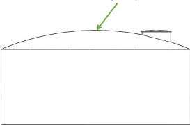
If installation must be along a curved dome surface, use the Domed Surface Install Kit to ensure sensor is level. 10 degree max angle of domed surface allowable.
