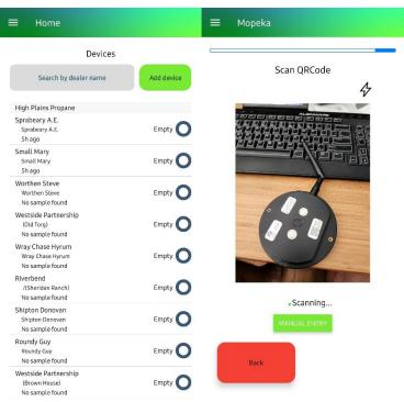
3. Scan QR code on sensor. The automated link in the QR code will open the Mopeka cloud to enter all the relevant information required, such as customer name, tank size, etc.
