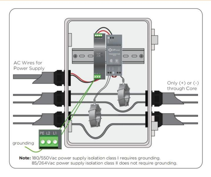
Note: Install the RSD-S-PLC before powering the Transmitter-PLC.
