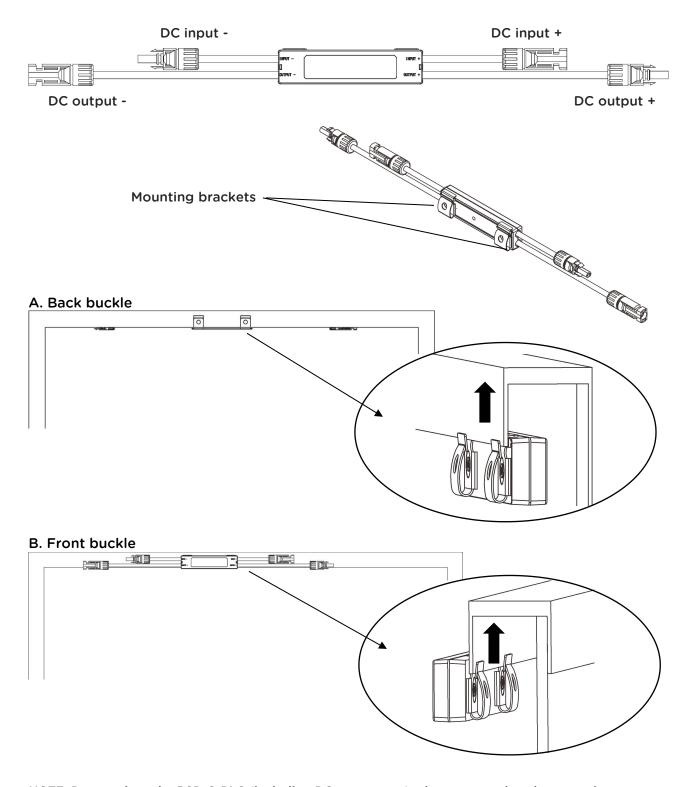
NOTE: Do not place the RSD-S-PLC (including DC connectors) where exposed to the sun, rain or snow, even gap between modules. Allow a minimum of 3/4"(1.5cm.) between the roof and the bottom of the RSD-S-PLC to allow proper air flow.
