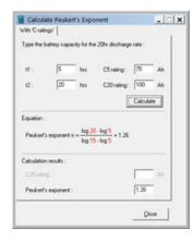
Please note that the Peukert exponent is no more than a rough approximation of reality, and that at very high currents, batteries will give even less capacity than predicted from a fixed exponent. We recommend not to change the default value in the battery monitor, except in case of lithium batteries.
