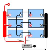
Always use busbars when applying midpoint voltage monitoring. The cables to the busbars must all have the same length.
