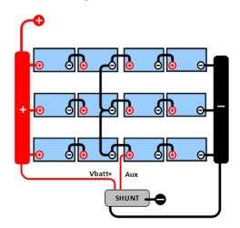
In an unmonitored battery bank the midpoints should not be interconnected, one bad battery bank can go unnoticed and could damage all other batteries.
