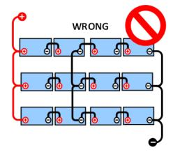
Due to the voltage drop over the positive and the negative cables the midpoint voltage are not identical.
