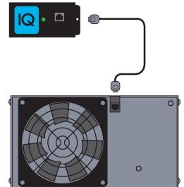
Note: External IOTA IQ Smart Charge Controllers are not compatible with DLS with internal IQ charge control. Current models are designed for 12V and 24V DC applications. Contact Customer Service for 48V options.
