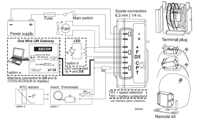
ATTENTION: If a longer connection cable is necessary, the cable cross section (or gauge) must be equal to or greater than the cable sizes recommended on the following table. Be careful that the input voltage at the appliance does not drop below the cut-out voltage of the compressor.
