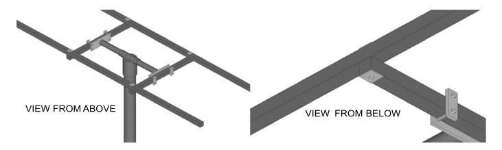
Place longitudinal tubes on top of cross pieces and bolt with square washers top and bottom as shown.
