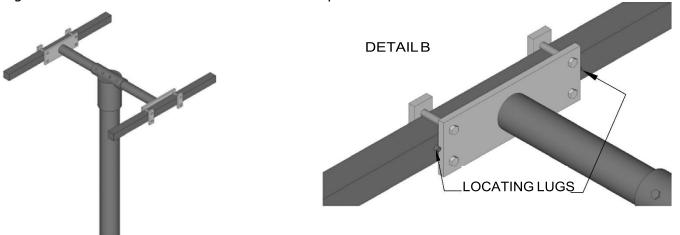
Slide cross pieces into flat bar arrangement. Make sure locating lugs on cross pieces are facing in. See Detail "B" of locating lugs.
