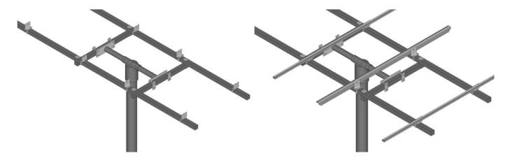
Attach aluminum angle brackets to longitudinals with smaller square U-Bolts and whiz flange nuts (bag #3). Oppose aluminum angle brackets as shown. Some mounts come with aluminum angle rails with punched holes for bolting on panels, and some come with aluminum extrusions which allow for panel attachment bolts or clips to slide in the "t-slot".
