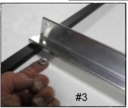
**For T-Slot Rails**: Lay T-Slot rails across the short axis of the panel as shown in Photo #1. Slide stainless bolts into T-slot of rail and position so they are opposite to the mounting holes on the frame
