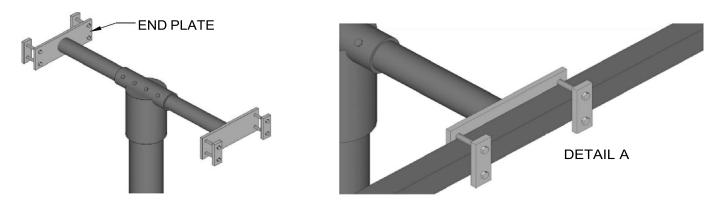
Finger tighten onto "Tee" end plates the aluminum flat bar and straight 1/2" bolts. Place entire "Tee" assembly on top of post. The aluminum flat bar and straight 1/2" bolts are shown in Detail "A". Tighten both set bolts and the four bolts on the top of the "Tee".
