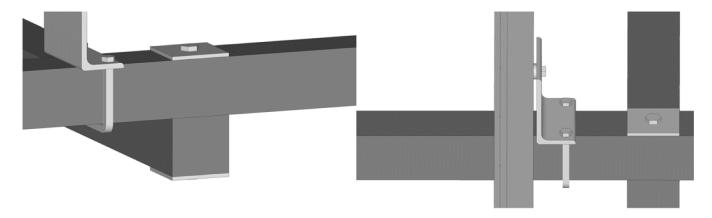
**General view of assembly**. When fastening panels to rails, place first panels at end of rails marked "TOP" and work down until all panels are in place with bolts finger tight. Cross measure array for square, check to see that all spaces (approx. ¼") between panels are equal, **then tighten** <u>all</u> **bolts**.
